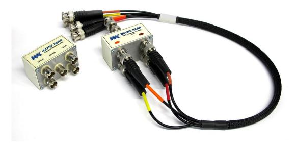
The 1J1001 4 to 1 BNC Converter is used to connect a Wayne Kerr 6500 analyzer to the Device Under Test using a single BNC connector. This is useful when the connection terminal of the DUT is a single BNC, such as some antennas. The outer of the single BNC is isolated.
